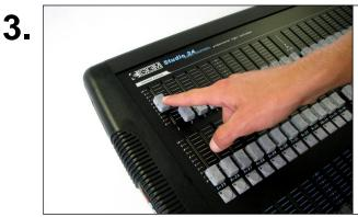
After you have used the Stage Flame, you must set it to safety mode again. You put the Stage Flame in safety mode by sliding shut the safety channel or setting it to a value outside the 40% to 60% range.
